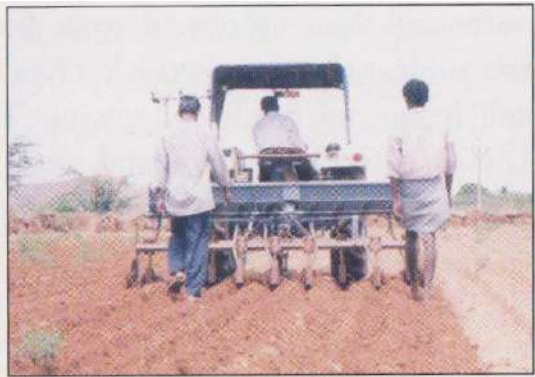
Tractor-drawn machine sowing of groundnut.
